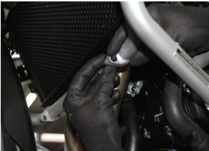
18. Tighten all four bolts to the recommended torque specs.
