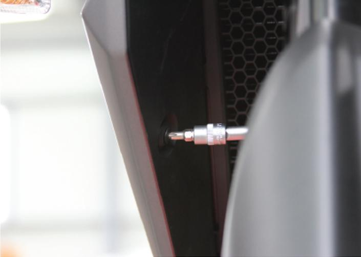
4. Using a 5mm Allen key remove the upper bolts. Again, from both right and left sides.
