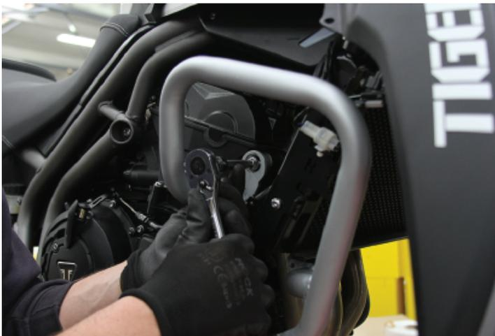
14. Insert the two M8 Allen bolts through the crash bar's lower mounting tab, thus connecting it with the engine guard. Put one washer on each of the two bolts and thread on the nyloc nuts. Gently tighten it.
