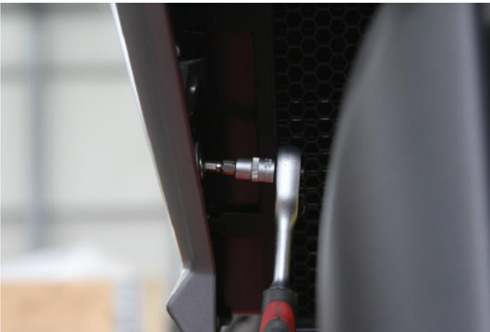
6. Carry on with the 5mm Allen key to remove the Allen bolt that is on the outside of the plastic fairing. Repeat on the left side as well.
