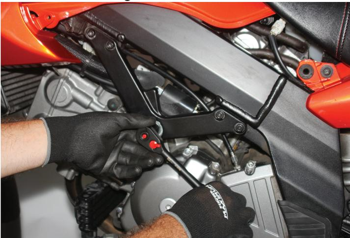
4. Put on the left side (rider's left) crash bar. Using a 6mm Allen, insert the two M8 fasteners into the top mount flange. Keep the fasteners slightly loose. Don't forget to apply threadlocker!
