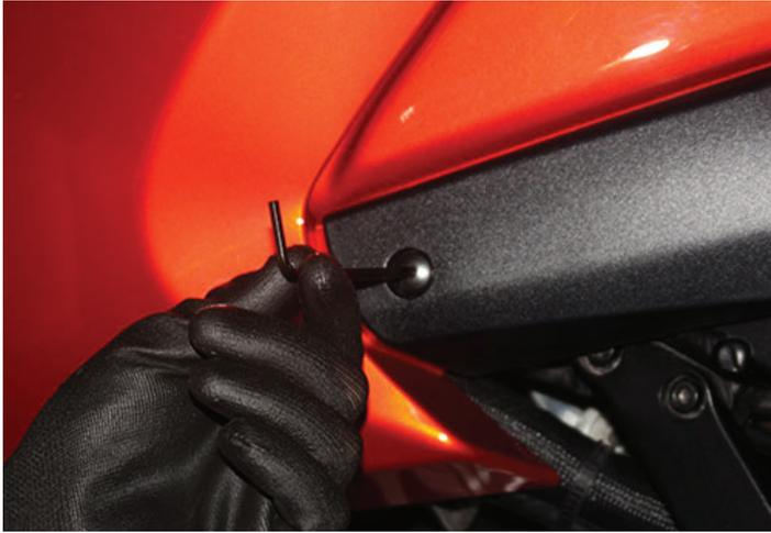
2. Use a 6mm Allen key to remove the top casting bolts on the left side where indicated.
