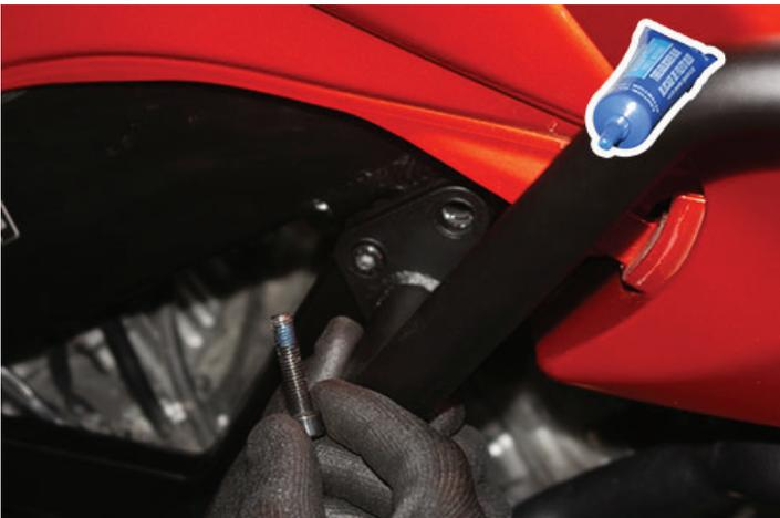
6. Place connector tube between the crash bars. Fasten both sides using four 6x16mm Allen head bolts, washers and nyloc nuts. Use 4mm Allen key and 10mm wrench. Do not fully tighten it, yet.
