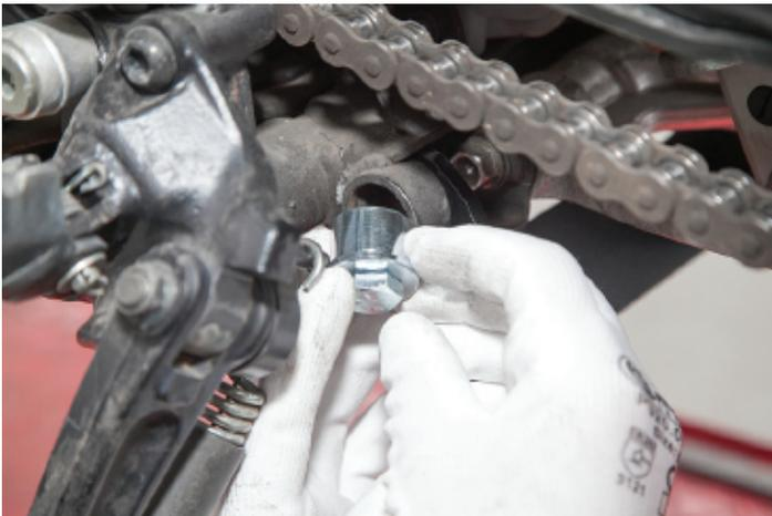
6. Push through the supplied 10mm diameter hex bolt with with the washer.
