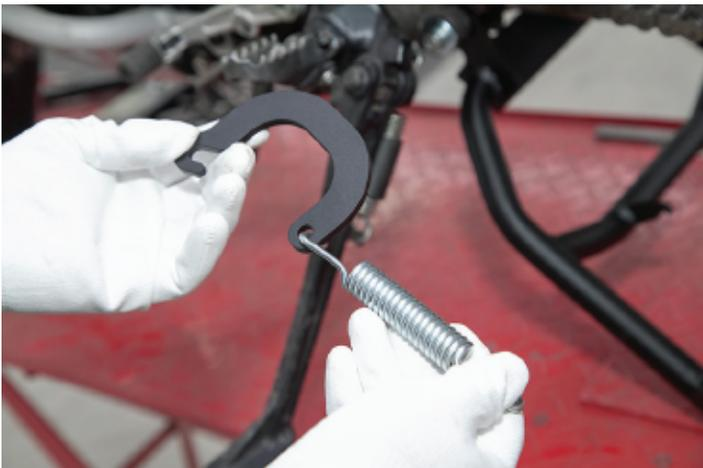
10. Attach the hook onto the mounting rod as shown in the photo.
