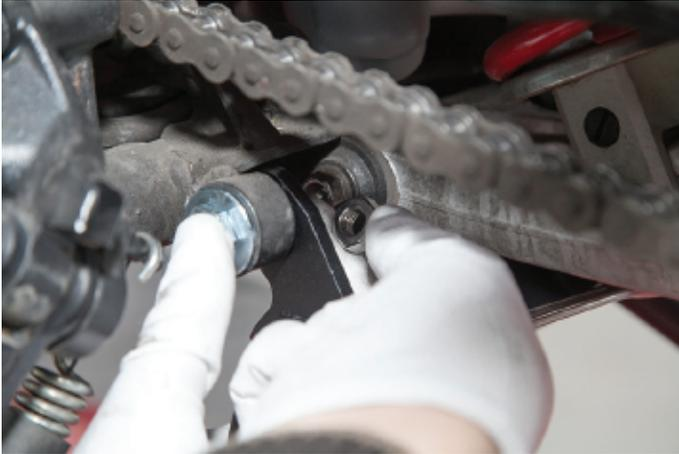
8. Using two 17mm wrenches tighten the bolt and locking nut.
