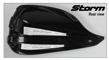
**NOTE**: Photos indicate correct placement of Drilling Templates on **REAR** of guard. Secure with clear tape prior to drilling.
